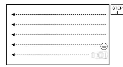
Start at wall closest to power outlet. Pull straight back without pushing down on handle.
